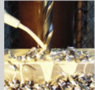
Chipbreaker drill in action
